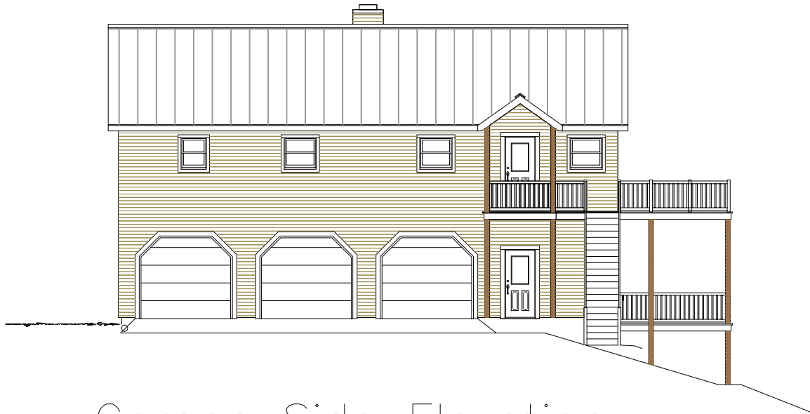
Garage Side Elevation
