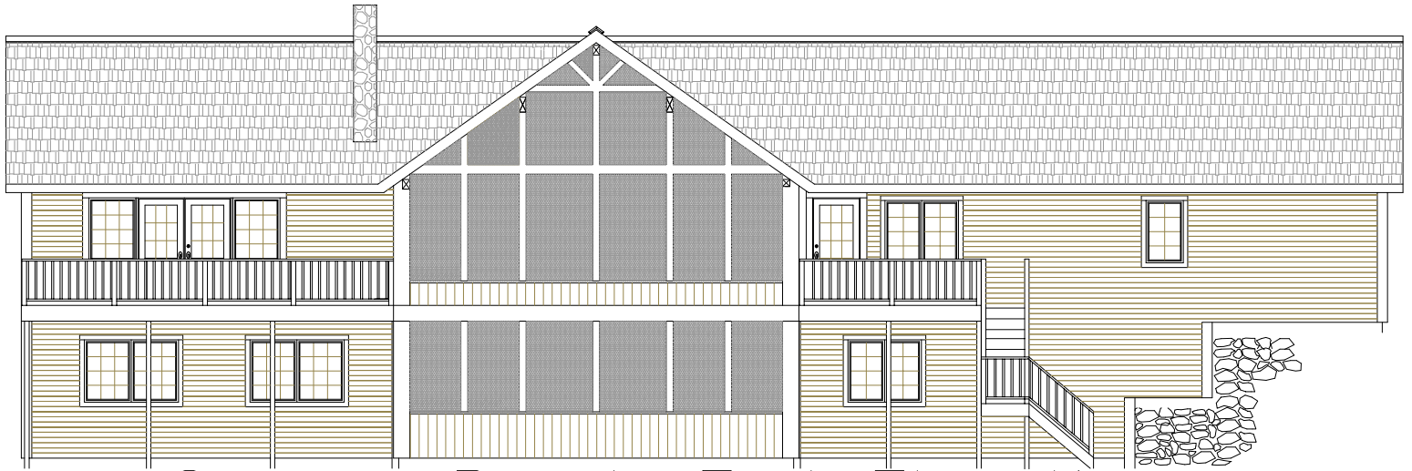
Screen Porch End Elevation
